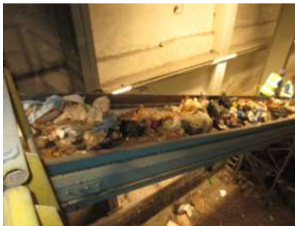
Image 10 – waste conveyor leading up to first magnetic separator
