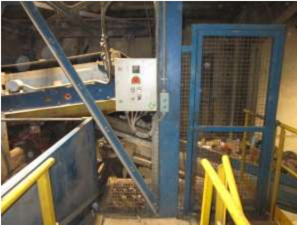
Image 40 – safety gate noted to be left open
