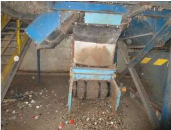
Image 42 – missing guarding over conveyor
