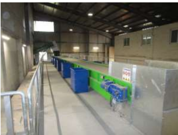
Image 46 – new machinery equipped with all guarding and signage
