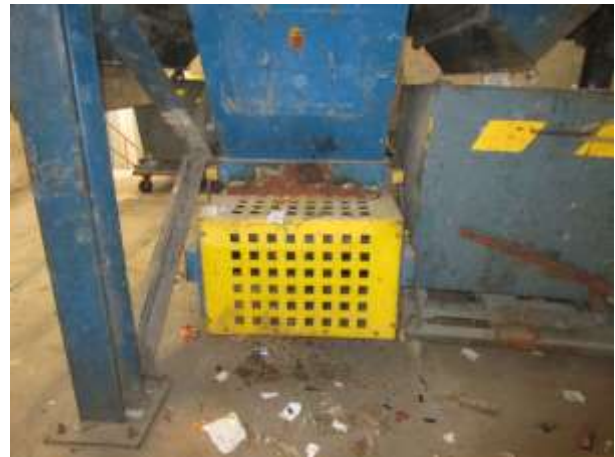
Image 43 – conveyor fixed guard in place
